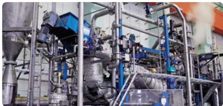
Inbicon thermal pretreatment pilot plants, 100 kg/h and 1000 kg/h
