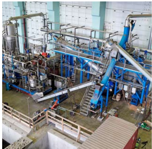
The pilot plant pretreatment process has a capacity of 1000 kg/ hour
